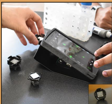
A multiplexed biomarker sensor that is quantified and read through a mobile phone for patient testing in clinical settings and even at home. Credit: Ozcan Lab at UCLA
