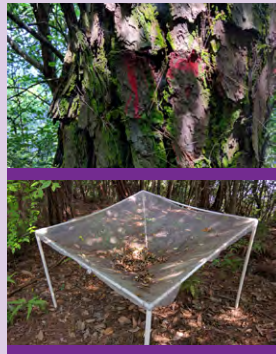
Top: A Pinus massoniana tree marked with a numbered tag and dendroband. Bottom: A litter trap for collecting fallen leaves on one of the TIL islands.
