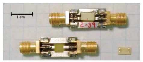
Multilayer low-pass microwave filter (2.5 GHz) fabricated from novel bismuth pyrochlore materials
