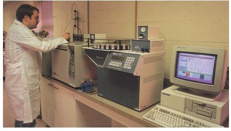
A student prepares a sample for analysis. The water content of a water-based coating will be analyzed using a Gas Chromatograph/Mass Spectrometer Head-Space Analyzer at EMU.
