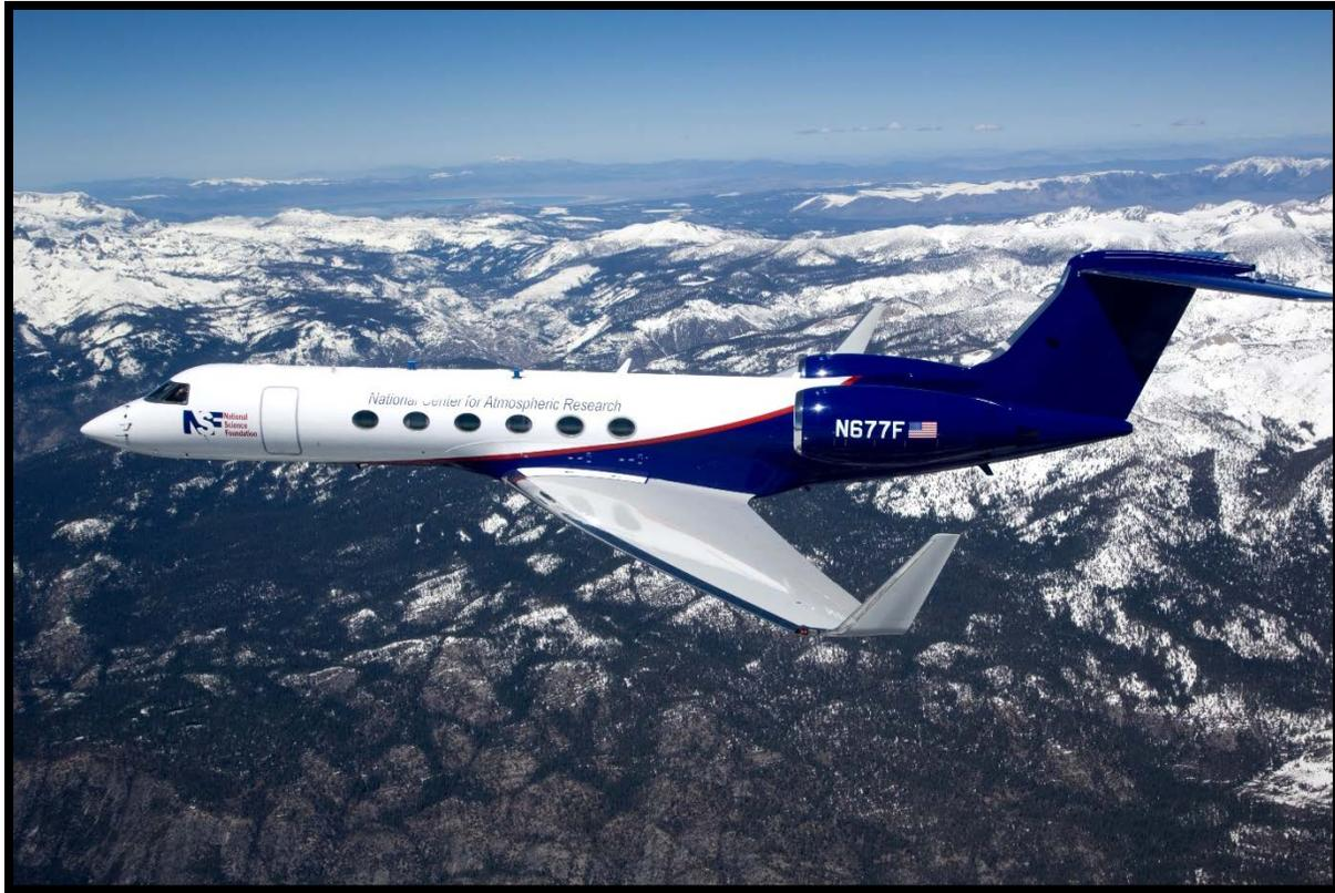
Figure 1. The HIAPER (High-Performance Instrumented Airborne Platform for Environmental Research), a modified Gulfstream-V aircraft owned by NSF and operated and maintained by NCAR. *Credit: © UCAR, by Clay Lacy Astrovision / Chad Slattery, licensed under a Creative Commons Attribution-Non-Commercial 4.0 International License, via OpenSky.*
