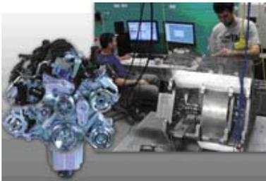
Right: specialized rotor test rig for evaluation of prototype absorbers. Left: V8 engine that could incorporate the absorbers, resulting in increased fuel efficiency. Credit: Brian Feeney, Michigan State University
