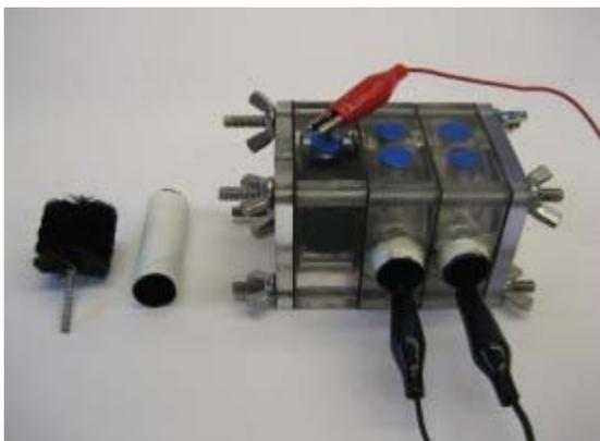
*Carbon brush anode, tubular cathode and fuel cell. Credit: Bruce Logan, Penn State.*
