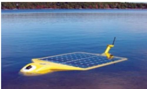
*The new solar-powered autonomous underwater vehicle (SAUV-II) will be used for a variety of environmental monitoring tasks. Credit: Arthur C. Sanderson, Rensselaer Polytechnic Institute; Richard Blidberg, Autonomous Undersea Systems Institute.*
