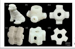
3D printed meso architectures via pressure-assisted binder jet
