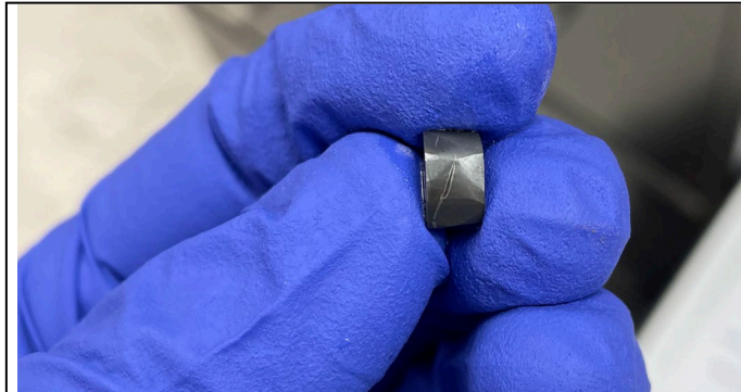
Spark plasma sintering of boron and carbon mixtures at 1930^\circ C. Handheld synthesized sample shown above
