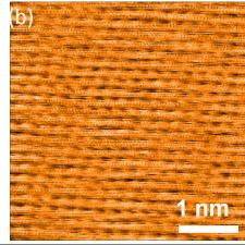
(a) Photograph of undergraduate students performing the scanning tunneling microscopy lab module developed by the PI for the College of Engineering at UW. (b) Image of the atomic structure of the surface of graphite acquired in the STM lab module.
