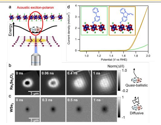
**Fig. 1.** (a) Schematic for optical far-field imaging of polaron transport. (b) stroboSCAT time series displaying exciton (dark contrast) and exciton-polaron (bright contrast) propagation in  $\text{Re}_6\text{Se}_8\text{Cl}_2$ . (c) Exciton propagation in bulk WSe<sub>2</sub>. (d) Linear sweep voltammograms showing catalytic water oxidation on surface-functionalized  $\text{Re}_6\text{Se}_8\text{Cl}_2$
