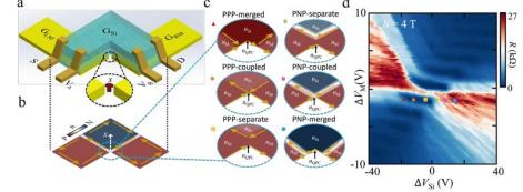
(a)(b) A novel quantum electronic device with dual-gated nanoconstriction, that allows (b) unprecedented control over quantum electronic states (c) and the resulting quantum phenomena.
