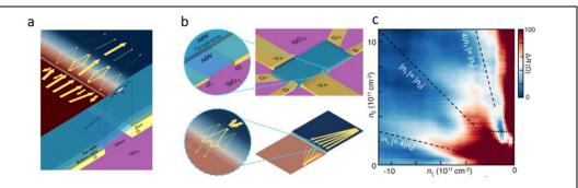
(a) A microcavity defined by carefully engineered local strain and electrostatic fields, creates (b) a controlled interference process for (c) effectively guiding electron flow towards desired direction.
