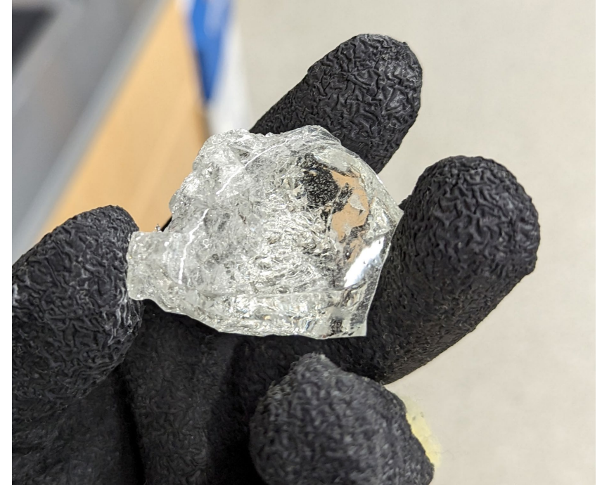
Piece of sodium aluminosilicate glass synthesized in the lab with a ratio of \text{Al}_2\text{O}_3/\text{Na}_2\text{O} = 1.17 .
