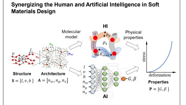
Workflow of HI and AI network design encoded by monomer projection length l, excluded volume v, and Kuhn length b of bare backbone and side chains, and network architecture  $A = [n_{sc}, n_g, n_x]$ . The network model is defined by the length of fully extended backbone,  $R_{max}$ , and effective backbone Kuhn length due to interactions between side chains,  $b_K$ .
