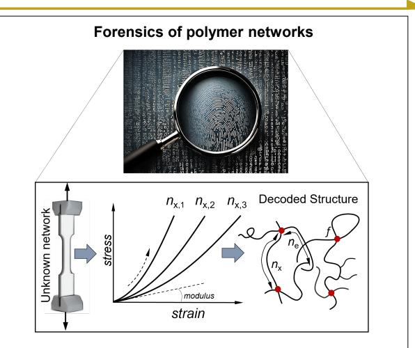
Schematics of network forensic approach based on the analysis of non-linear response of elastomers to deformation.
