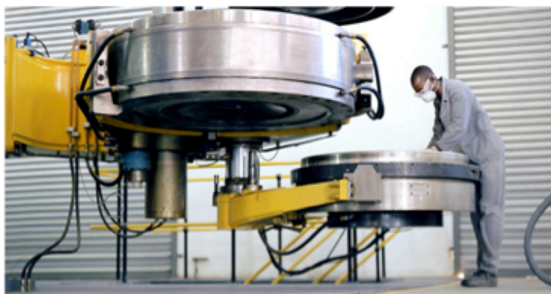
Figure 3.1.5. (a) high-pressure apparatus. (b) 15 carat diamond anvil produced by CVD compared to a conventional 0.3 carat natural diamond anvil (courtesy of R. Boehler, Oak Ridge National Laboratory).
