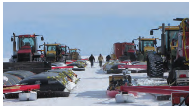
Long-distance, over-snow, heavy-haul traverse trains provide an efficient alternative to airlift for moving cargo, fuel, and science equipment to remote sites. Credit: The Whillans Ice Stream Sub-glacial Access Research Drilling Project
