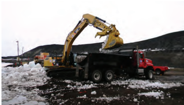
The USAP recently introduced more versatile dump trucks at McMurdo Station. These multi-purpose, commercial trucks have beds that can be converted for varied uses such as for towing, cargo movement, and hauling bulk materials. This reduces the types and numbers of vehicles required and capitalizes on the savings to be gained from standardization. Credit: Martin Reed, Antarctic Support Contract
