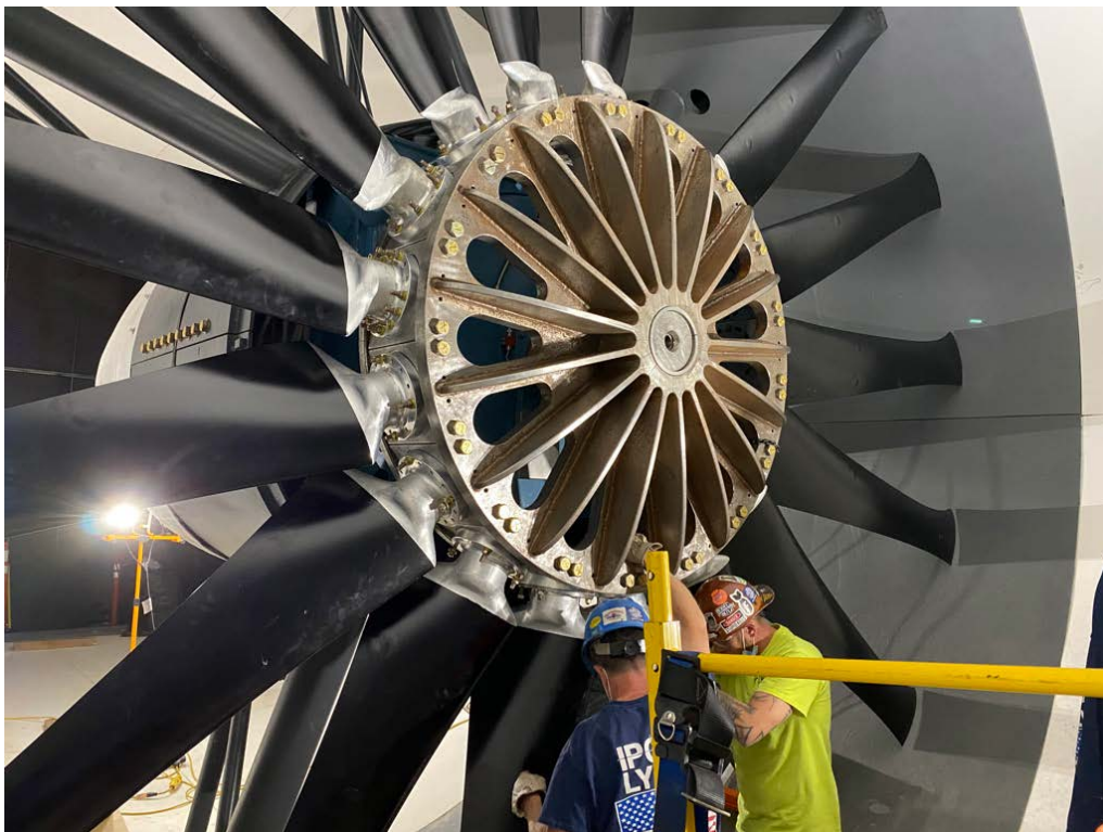
Figure 2: Aerolab MIT Fan During Assembly
