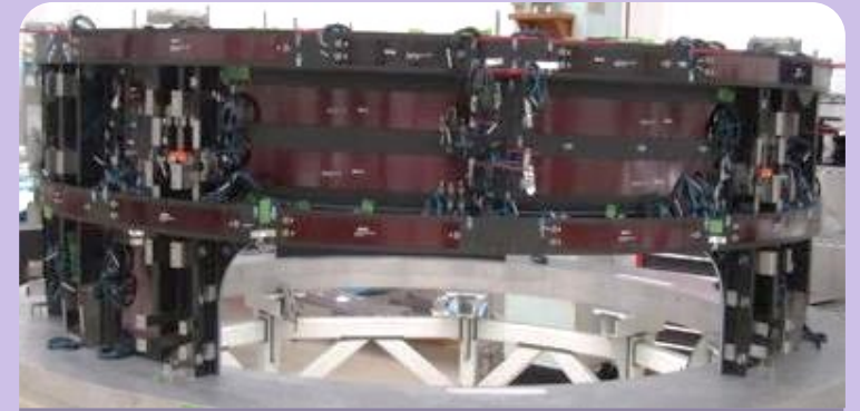
Forward Metering Shell w/thermal control hardware installed
