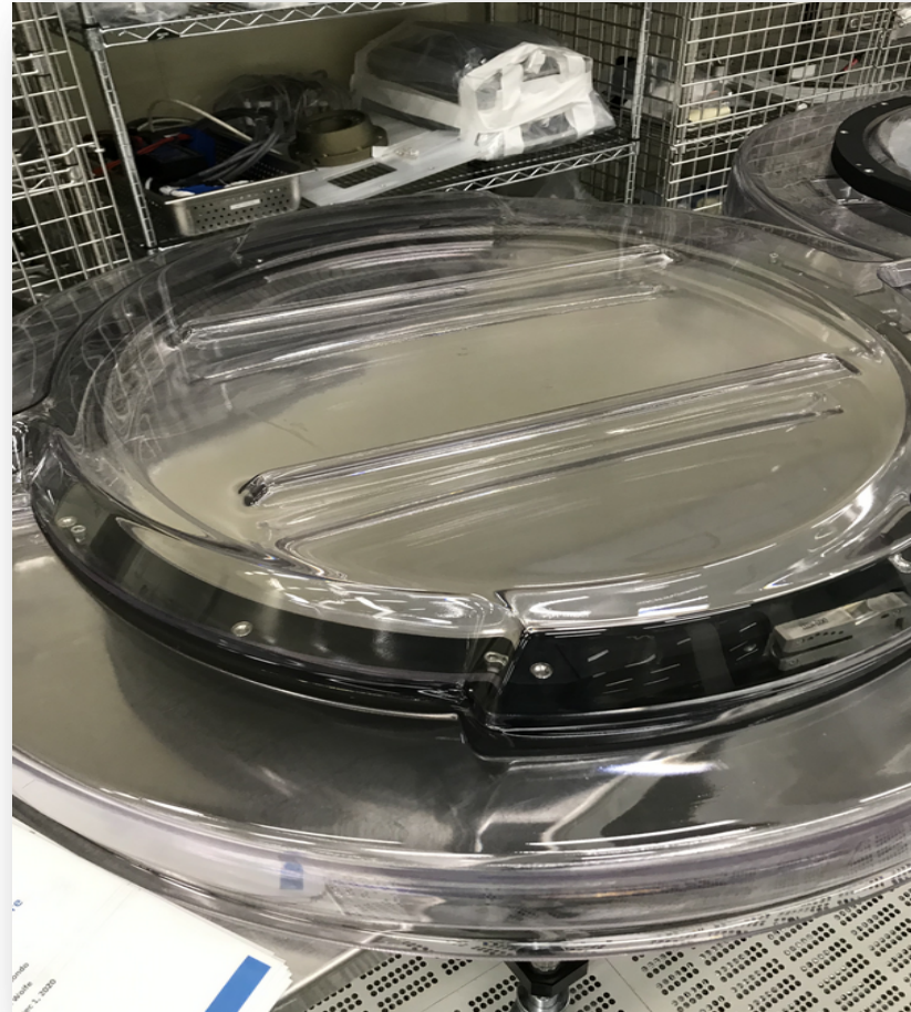
y-band filter in its inner container prior to final packing at LLNL.
