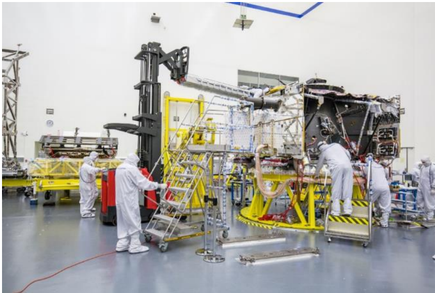
Second sunshield mid-boom installation
