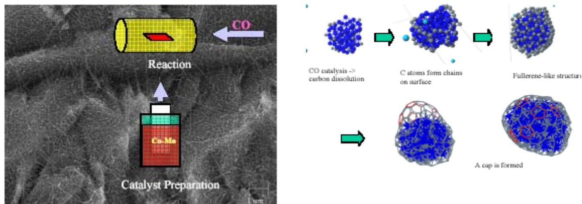
Smart manufacturing of materials is enabled by a molecular dynamic simulation of the reactive force fields that predicts the material properties and the synthesis pathway. Growth of single walled carbon nanotubes (shown extending over a surface) can be controlled to conform to specific technological requirements (size and chirality) by using precisely defined nanoscale catalytic particles. (Balbuena and Resasco, Texas A&M University and University of Oklahoma)
