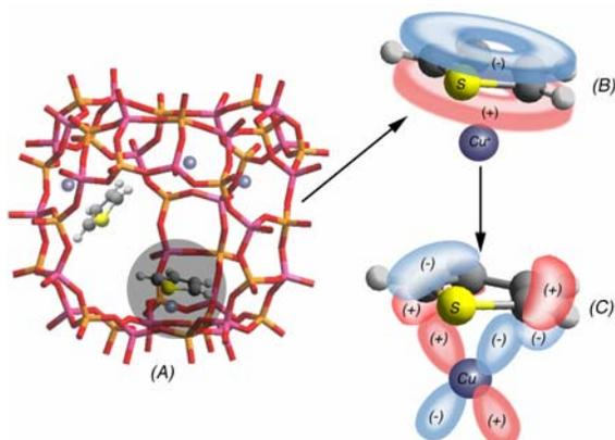
Selective adsorption of sulfur from fuels: (A) zeolite cage for trapping sulfur, (B,C) details of copper's role in maintaining the special electronic structure for sulfur trapping. Removal of contaminants will reduce the air pollution resulting from burning sulfur- and nitrogen-containing compounds. It may also solve the critical problem involved in using liquid fuels as the power source for future hydrogen fuel cells, which are degraded by sulfur contamination. (Yang, University of Michigan)
