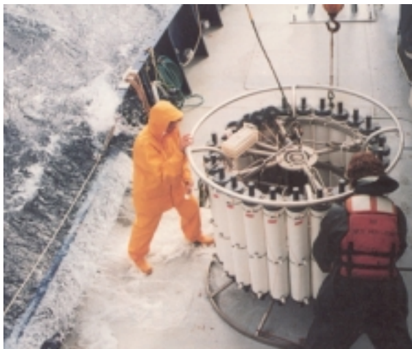
Deployment of a CTD (Conductivity/Temperature/Depth) rosette from R/V New Horizon. Photo courtesy of Scripps Inst. of Oceanography Explorations, La Jolla, CA.
