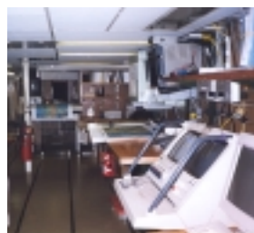
Underway ocean floor swath mapping capability is provided by a 90° multibeam bathymetric mapping system
