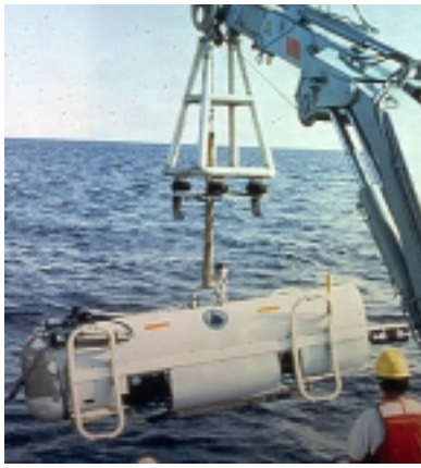
A DSL-120 sonar vehicle. Photo courtesy of WHOI, Woods Hole, MA.
