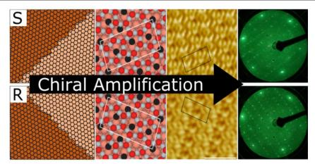
A small degree of chirality induced by slight misorientation of a metal surface (1 site/20 nm<sup>2</sup>) is amplified by oxidation to yield a homochiral oxide with a dense regular array of chiral oxide pores (~75 sites/ 20 nm<sup>2</sup>).
