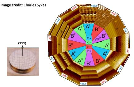
Collage of data showing how the local orientation of a custom-made domed Cu(111) single crystal dictates the local orientation and chirality of the '29' oxide. A chart in the center shows the different oxide orientations and chiralities at different locations around the dome.
